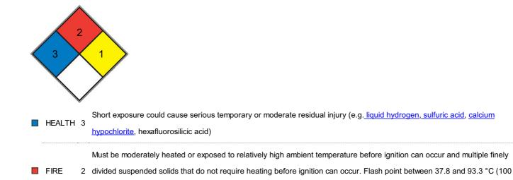
REACT 1 Normally stable, but can become unstable at elevated temperatures and pressures (e.g. <u>propene</u>)
