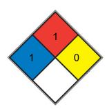
HEALTH 1 Exposure would cause irritation with only minor residual injury (e.g. <u>acetone</u>, sodium bromate, potassium chloride)
